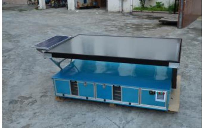
Model (shown on work table) with solar air collector set at 30 degrees. This setting is suitable for temperate latitudes. The setting of the collector can be easily adjusted between 20° and 45° for the seasonal changes of solar angle or for various latitudes.
